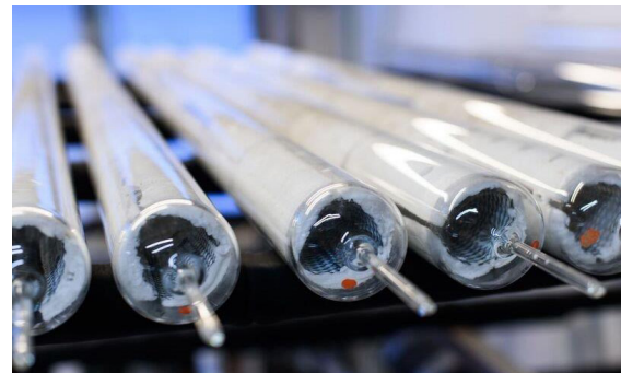
SaltX reactor with nano-coated salt
