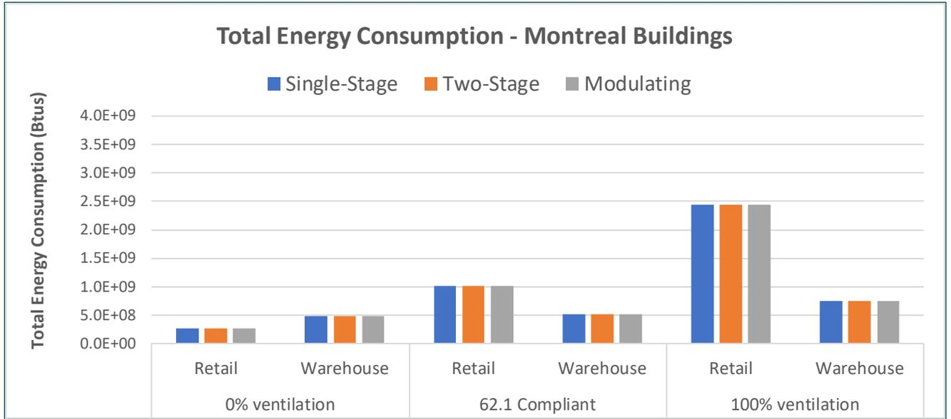
Figure 8: Total Energy Consumption Outputs from Baseline Simulations – Climate Zone 6 (Montreal)
