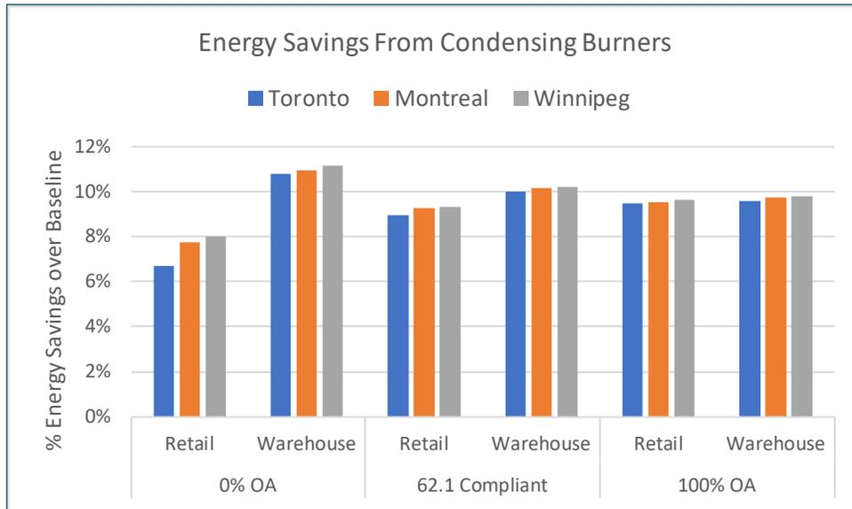
**Figure 14: Modeled Energy Savings – Condensing Burners**
