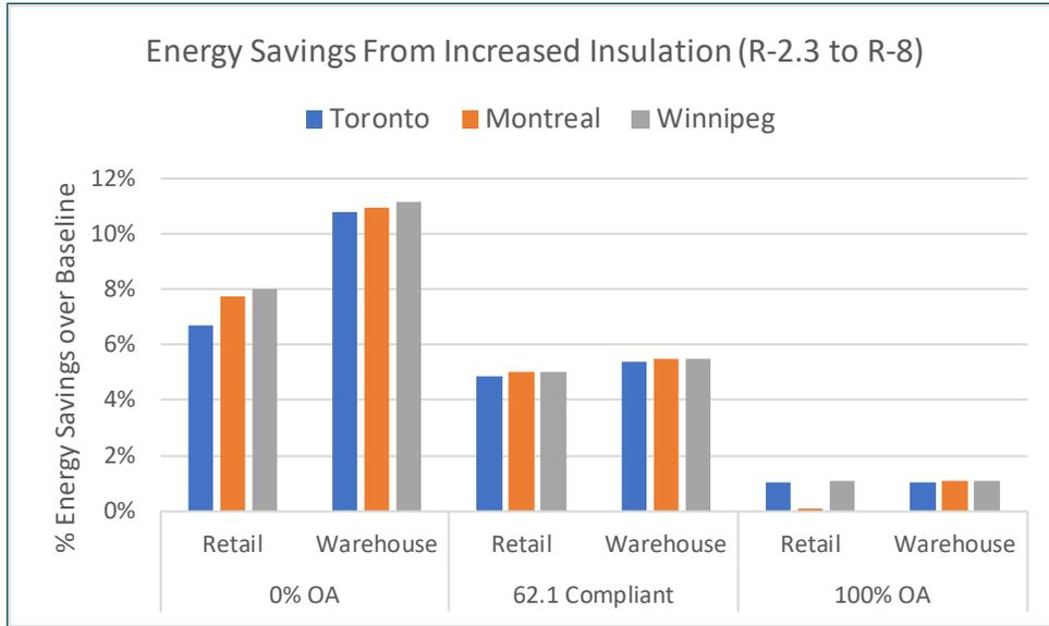
Figure 12: Modeled Energy Savings – Increased Enclosure Insulation
