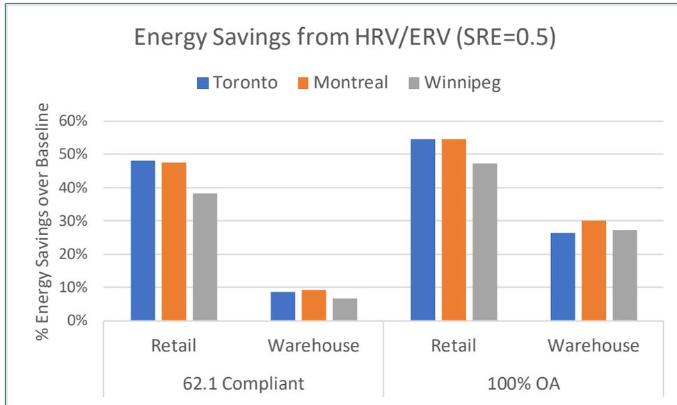
**Figure 15: Modeled Energy Savings – Heat Recovery Ventilation**
