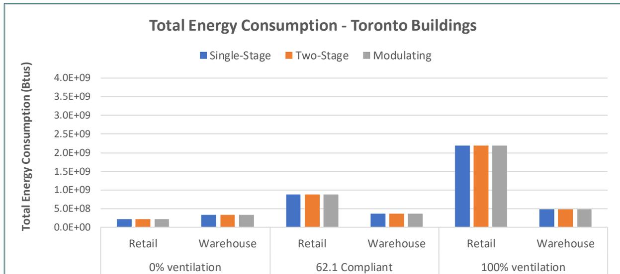
Figure 7: Total Energy Consumption Outputs from Baseline Simulations – Climate Zone 5 (Toronto)
