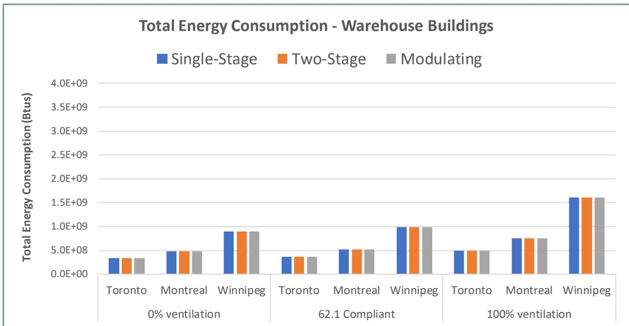
Figure 11: Total Energy Consumption Outputs from Baseline Simulations – Warehouse Buildings
