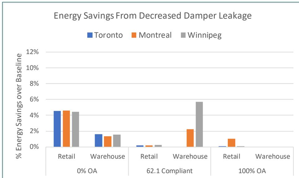
Figure 13: Modeled Energy Savings – Decreased Damper Leakage
