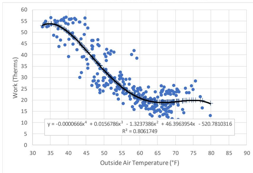
Figure 31 shows the relationship between heat pump performance and the daily average outside air temperature (ambient to the GAHP-A units).
