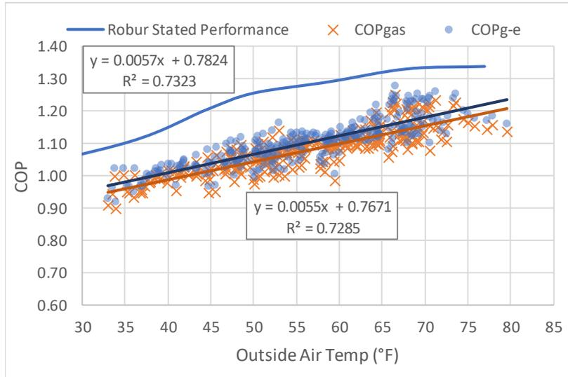
Figure 37 shows the daily spread of COP<sub>gas</sub> by month and the corresponding average outside air temperature during that month.
