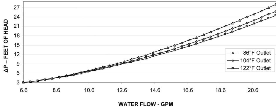
**PRESSURE DROP - Heating mode ( $\Delta P$  condenser / absorber)**
