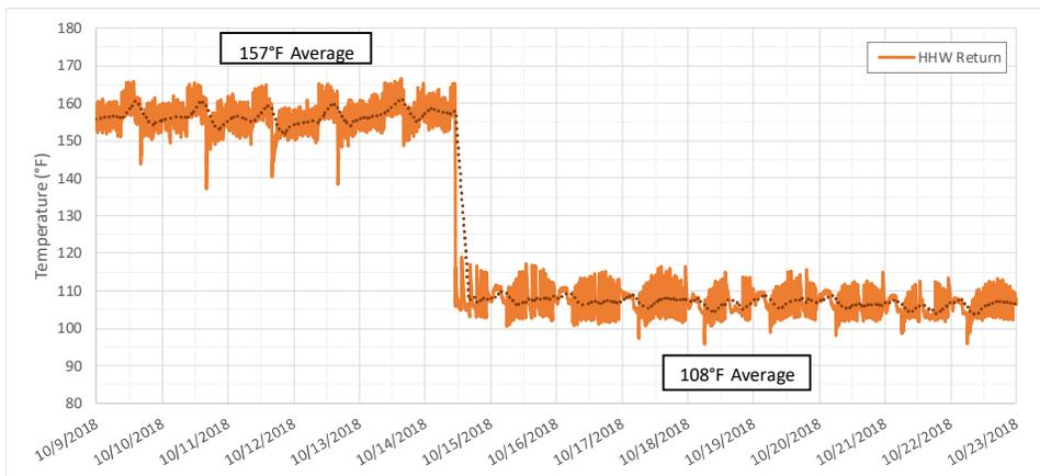
The addition of VFDs on the DHW water heater pumps and an EC smart pump on the building circulation loop resulted in a 10°F reduction in average DHW return temperature, and the average HHW loop temperature was reduced by nearly 50°F. The DHW and HHW return temperature reductions in Phase 1 enabled the GAHP-A units with supply temperatures between 120-140°F to transfer heat to both loops most of the time.
