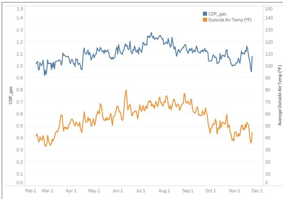
Table 11 shows the performance results from the performance period, which was between 2/14/2019 and 11/24/2019. On average the GAHP-A system delivered 98,178 Btu/hr which represents a system utilization of 39.7% based on the nominal capacity of 123,500 Btu/hr for each of the two units. On the coldest days of the performance period (<40°F), the units consistently delivered 190,000 Btu/hr, indicating both units operated over 18 hours in a 24-hour period (76.9% utilization).
