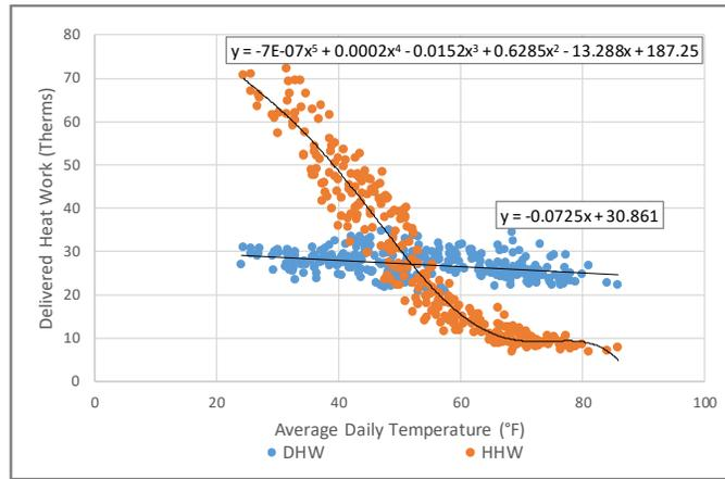
By applying the DHW and HHW regressions shown in Figure 28 to typical meteorological year (TMY3<sup>6</sup>) average daily dry-bulb temperatures, an annual hot water load profile was generated for the site. Figure 29 shows the daily load to the facility over a typical weather year.
