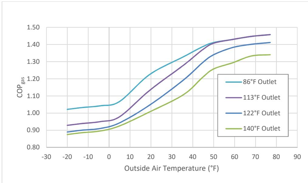
FIGURE 42 - GAHP-A OUTPUT CAPACITY CURVES
