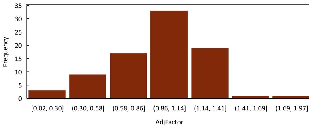
**Figure 13: Histogram of Adjustment Factor, Constant Speed Pumps**
