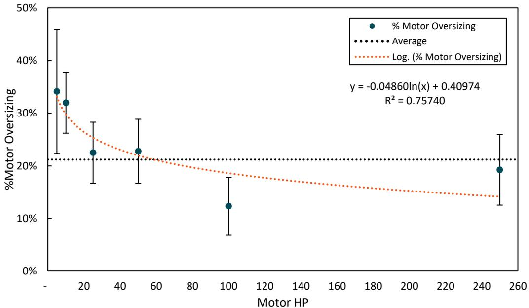
**Figure 1: Motor Oversizing vs Motor HP**
