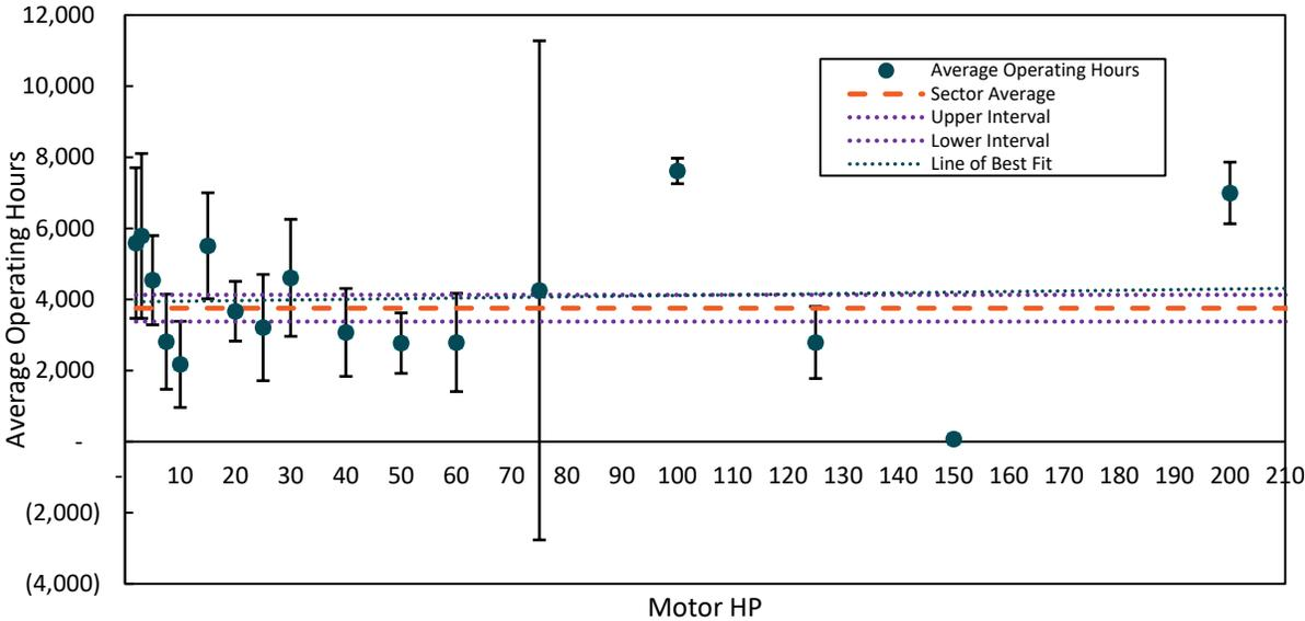
**Figure 6: Average Commercial HVAC and DHW Operating Hours, by Motor HP**
