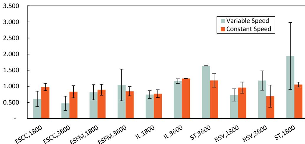
**Figure 15: Adjustment Factor by Pump Class and Nominal Speed**
