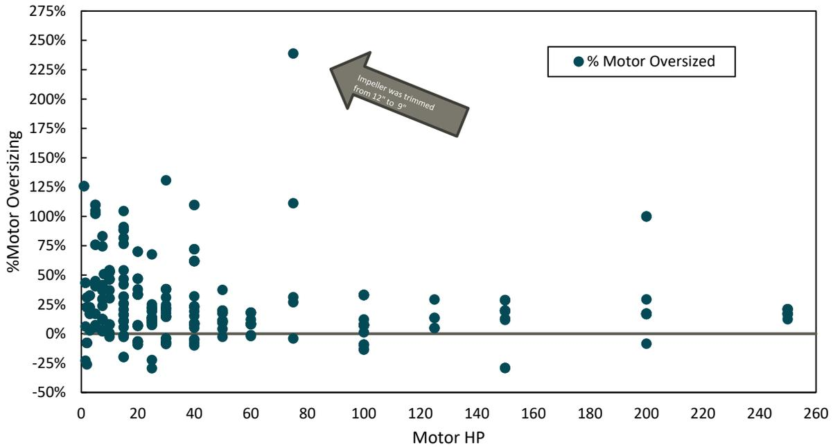
**Figure 18: Percent Motor Oversizing vs Motor HP**
