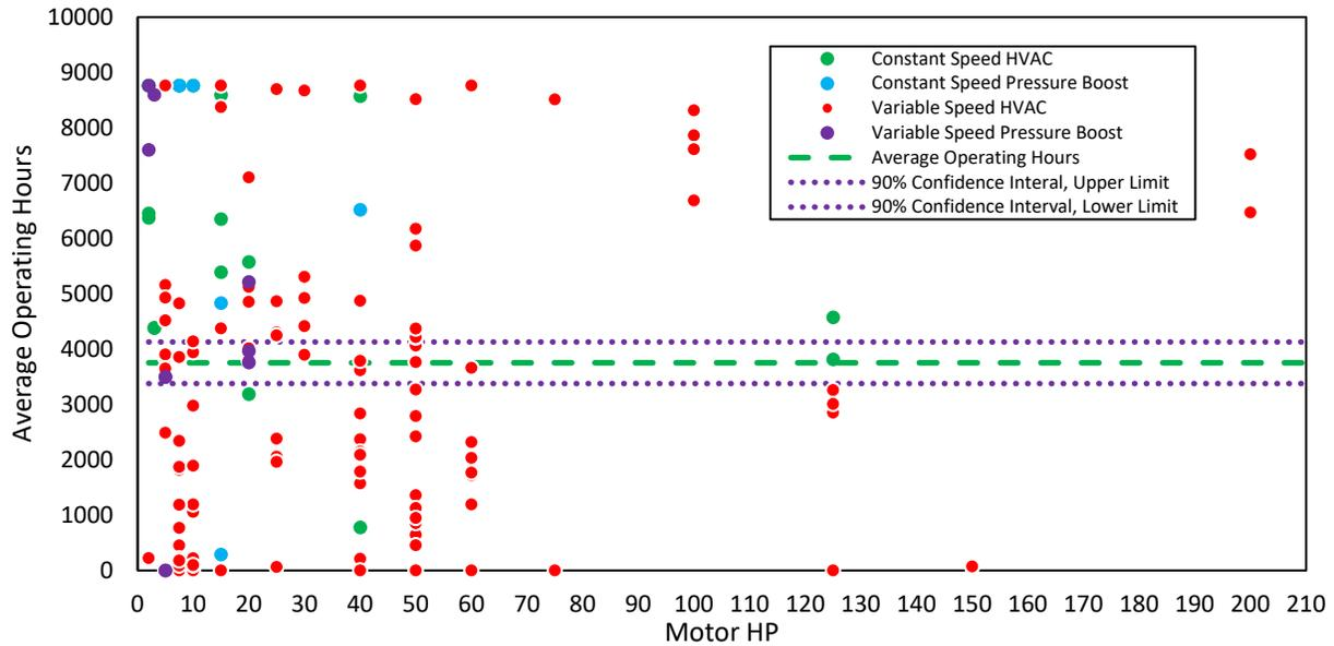
**Figure 7: 'Commercial HVAC and DHW' Operating Hours, by motor HP**
