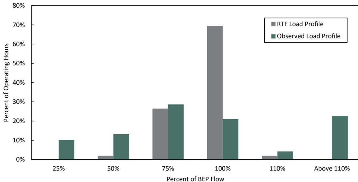
**Figure 21: Constant Speed Load Profile, Observed and RTF Estimated**
