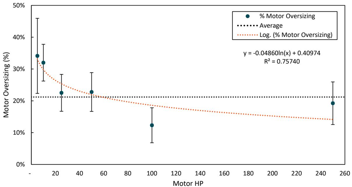
**Figure 19: Percent Motor Oversizing vs Motor HP, by Motor HP Bin**
