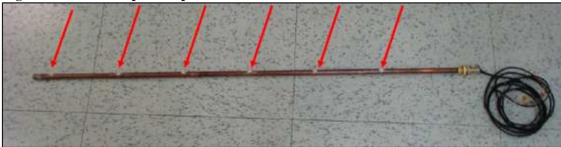
Figure 3. Thermocouple Temperature Tree
