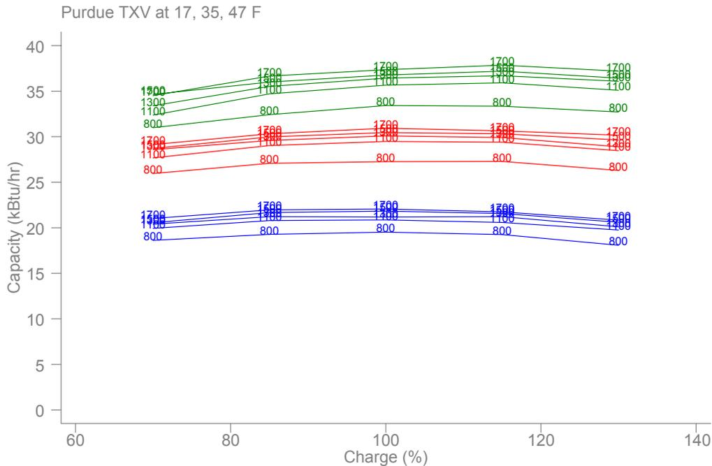
**Figure 52. Capacity (TXV) versus Charge at three outdoor temperatures**
