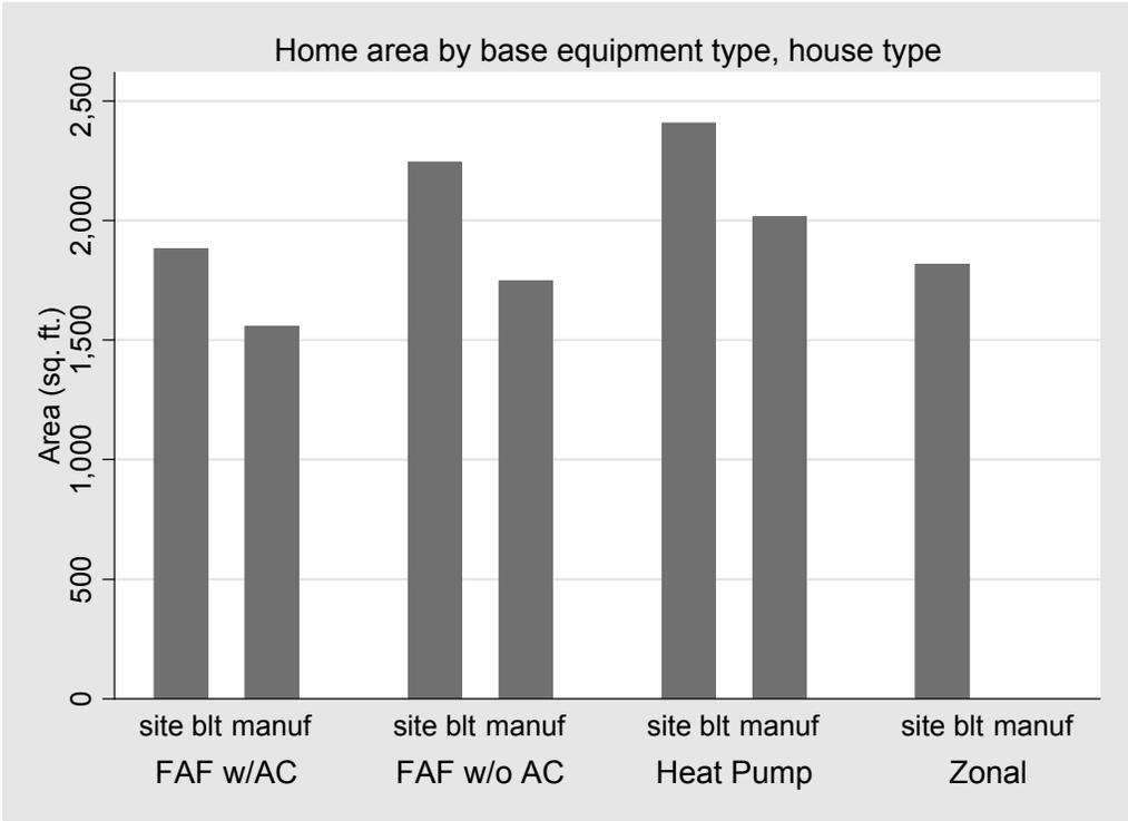
**Figure 11. Building Size by System Type (N=470)**
