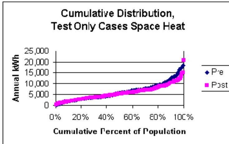
**Figure 21. Distribution Profile of Space Heat Consumption**
