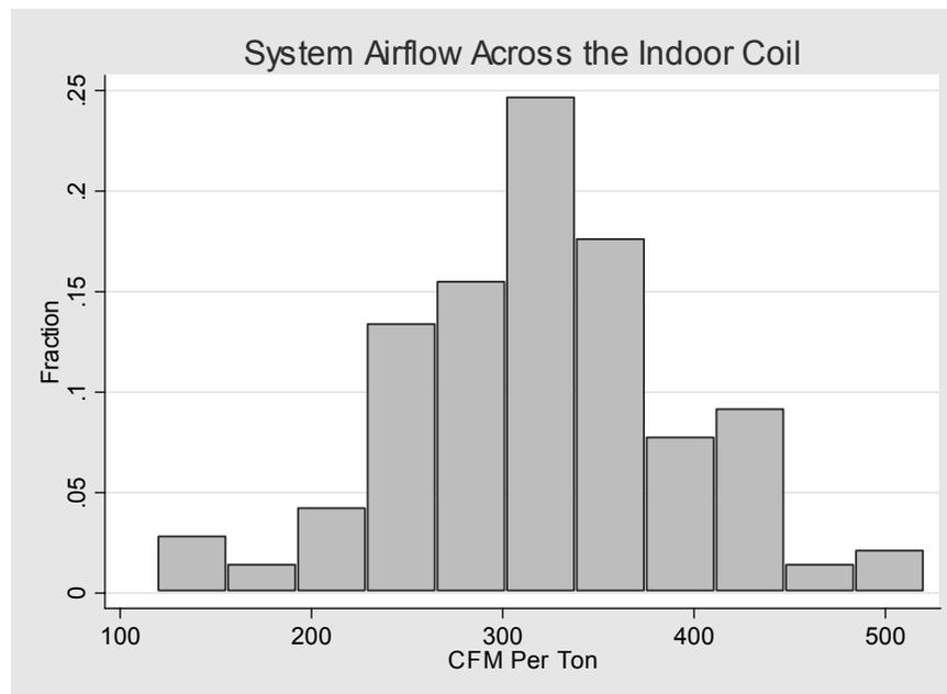
**Figure 38. System Airflow Distribution**
