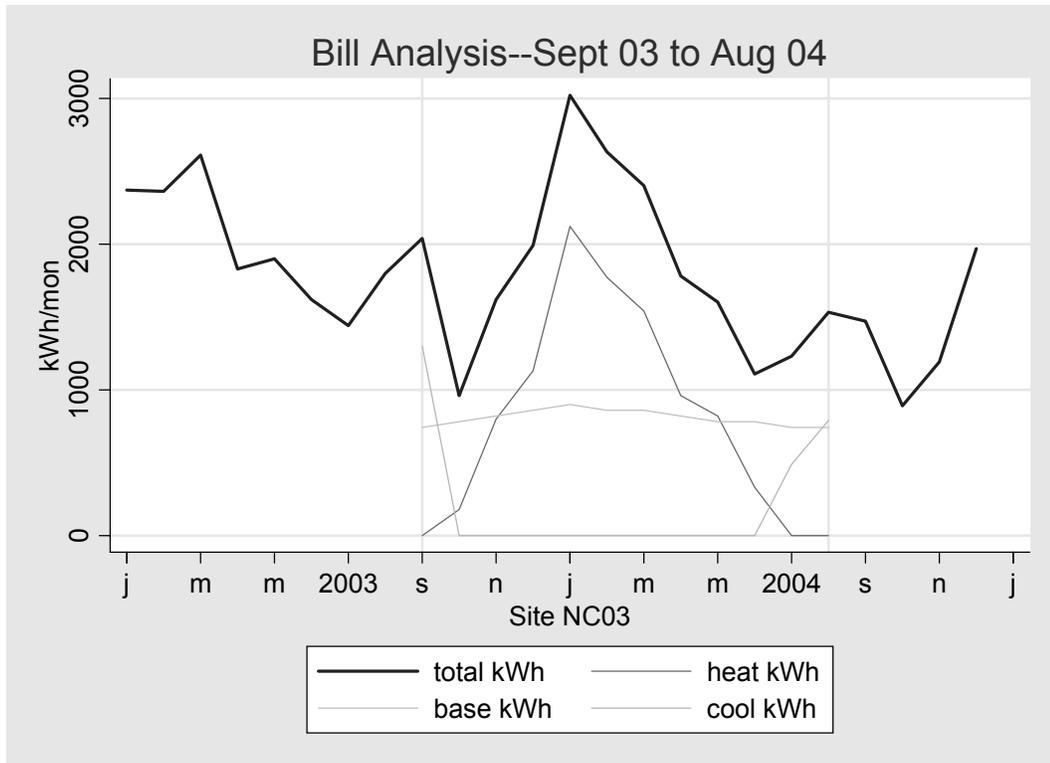
**Figure 48. Distribution of Consumption by Load Type**
