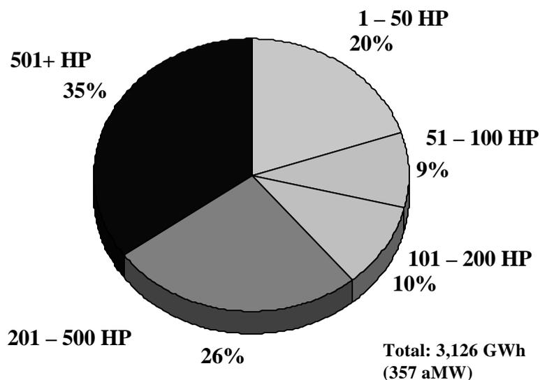
The installed base of pumps in the pulp and paper industry range from 1 to greater the 500 HP, with a substantial concentration of 1-50 HP pumps. However the greatest consumer of pump energy are the pumps greater than 500 HP in spite of the fact that these pumps have the lowest installed base in the pulp and paper industry.
