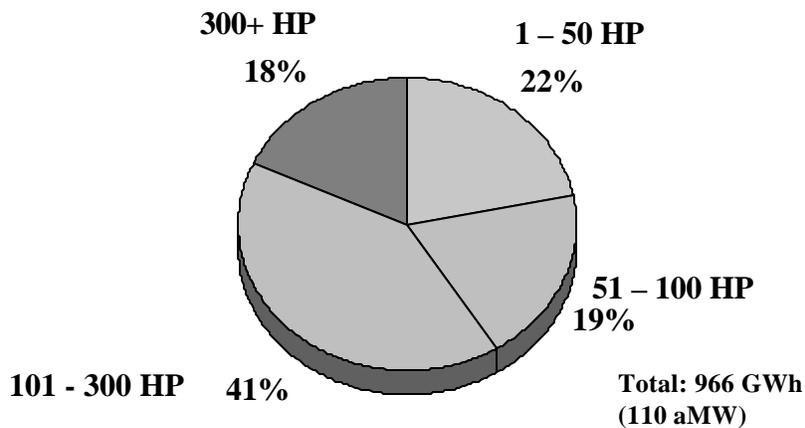
The different size HP pumps in the water and wastewater treatment consume disproportionate amounts of energy. Although 50 HP make up 63% of the pumps installed in the facilities, they consume relatively little energy. Only 22% of pump energy in the water and wastewater industries is from 1-50 HP motors. On the other hand, pumps in water and wastewater treatment plants greater than 300 HP make up only 3% of installed pumps but account for 18% of consumed pump energy.
