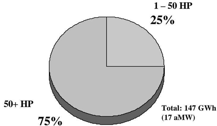
Fans and blowers in the water and wastewater treatment facilities vary in size. A majority (57%) of fans and blowers installed in facilities are less than 50 HP. However, fans and blowers under 50 HP in water and wastewater treatment plants account for 25% of the fan and blower energy consumed.
