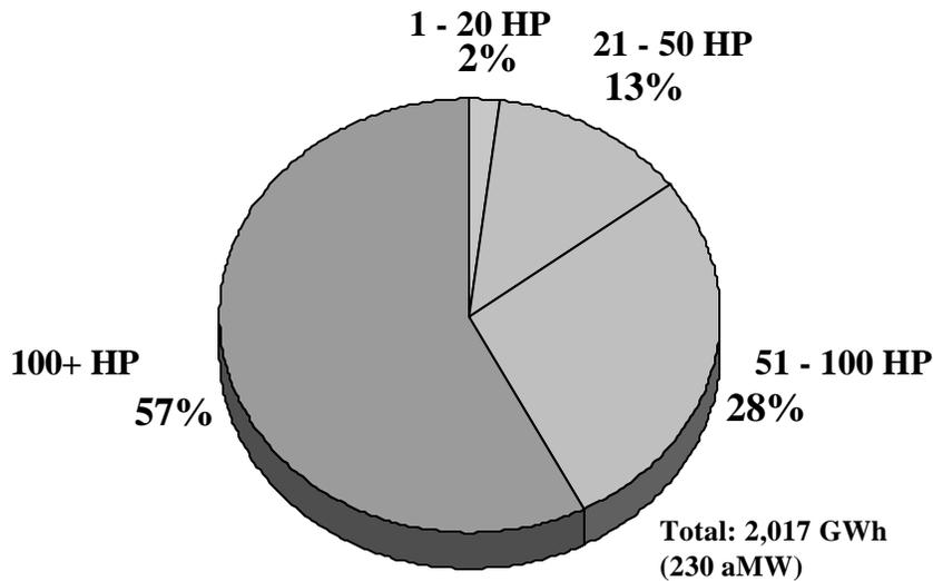
The installed base of fans and blowers in the pulp and paper industry range from 1 to greater than 100 HP, with a relatively even range of installed base distribution among HP ranges. However the greatest consumer of fan and blower energy are the fans and blowers greater than 100 HP, which consume 57% of fan and blower energy consumed.
