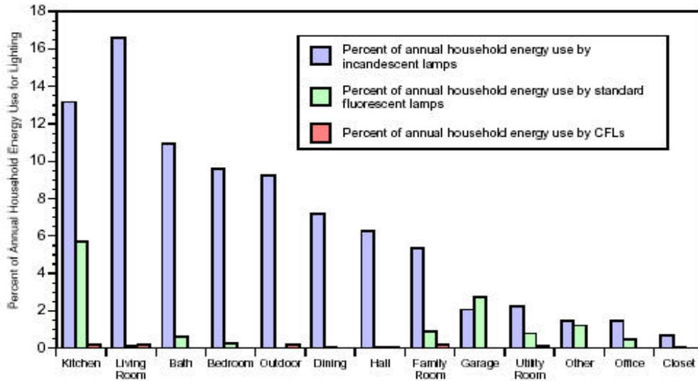
Note: The data for incandescent lamps also includes other lamp types including quartz and some HID lamps; these "other" lamp types, however, account for less than 1% of the energy consumption represented by the "incandescent" category in the figure. Data were obtained from TPU analysis of lighting energy use in 161 single-family homes in the Pacific Northwest between 1993 and 1995. Rooms are listed in order of decreasing energy consumption.
