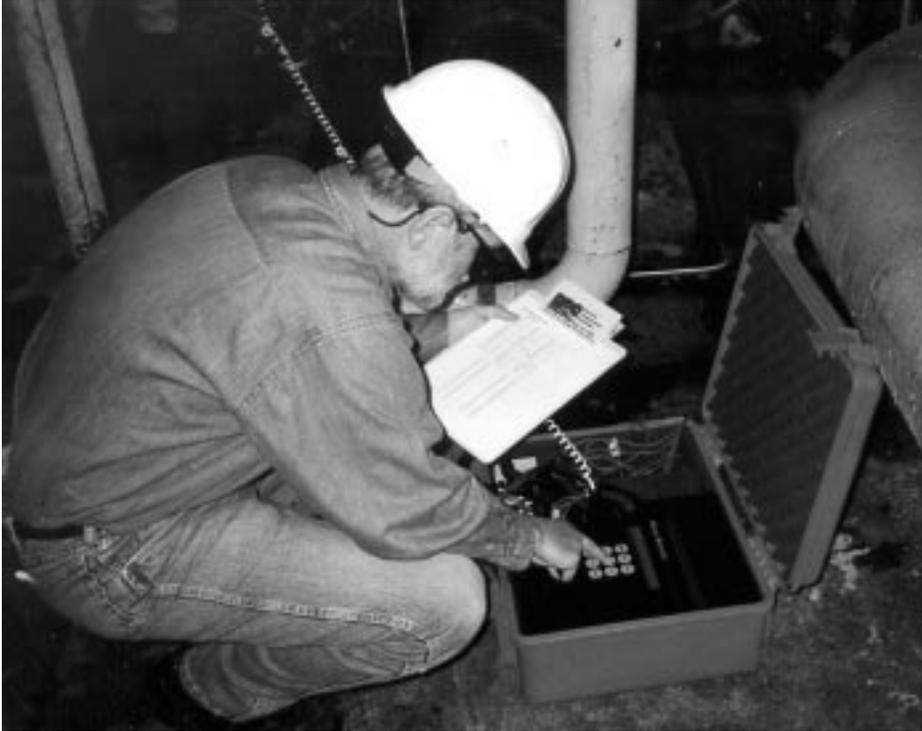
During the dry run WSU staff indeed made an error. This possibility was anticipated and it was the reason for having a dry run first. Some of the nameplate data was entered after one of the readings was taken. That caused the winding resistance to be readjusted by the machine, which led to an erroneous result. Once we detected the error, the manufacturer was able to back calculate the correct result for us.
