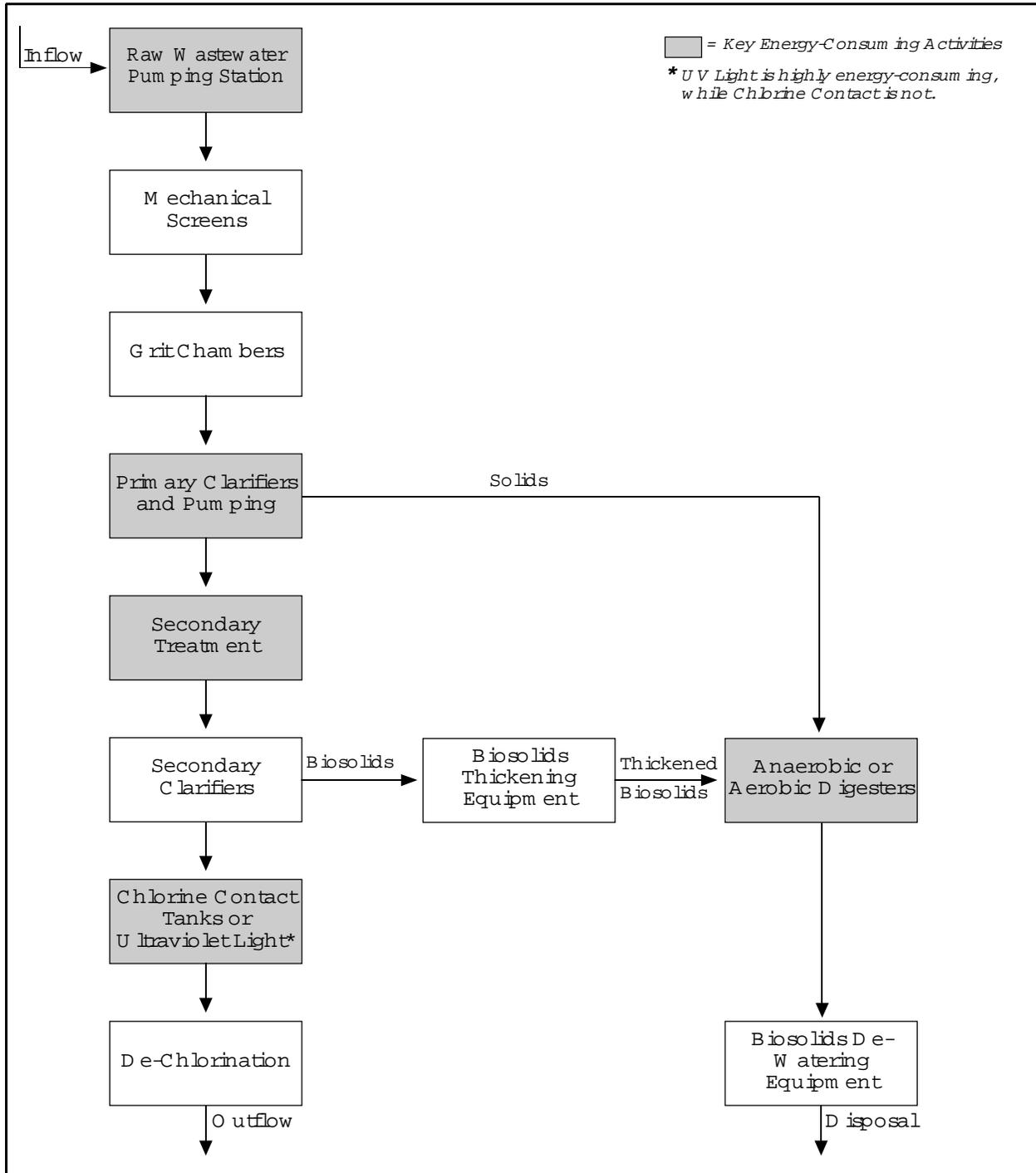
Activated sludge processes involve two components: biological conversion and solids separation. Biological conversion entails the decomposition of organic matter within the wastewater stream. Solids are then 'settled' and removed before the water is discharged for release or further treatment.
