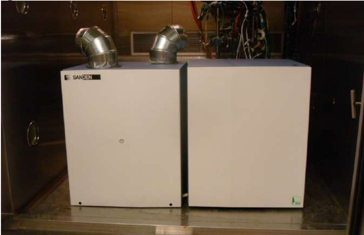
Figure 1. HPWH Test Unit Installed Inside Thermal Chamber
