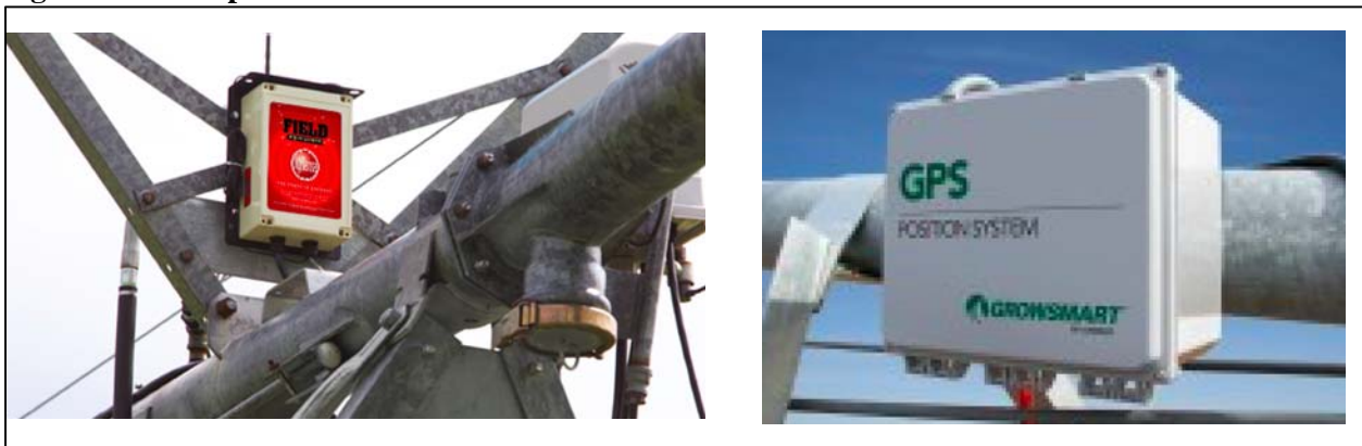
Figure 12. Examples of Pivot Controllers Mounted onto a Pivot
