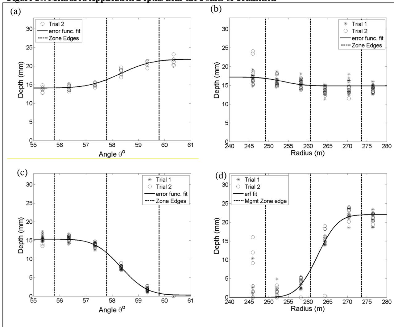
Notes: (a) transition from 50% to 80%, (b) transition from 60% to 50%, (c) transition from 60% to 0%, and (d) transition from 0% to 80%. The solid black lines are the empirical fits (using nonlinear least square optimization). Dashed lines are the boundaries between management zones.
