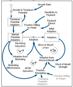
Figure 8. Flow Diagram of Diffusion Model
