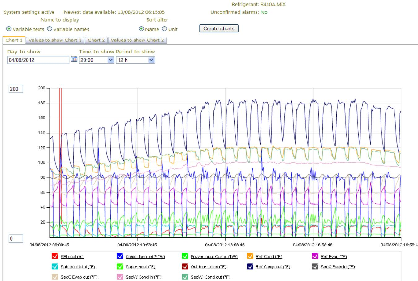
**Figure 9, RTU1 operates with on-off and does not reach stable operation even on a 100° day (°F)**
