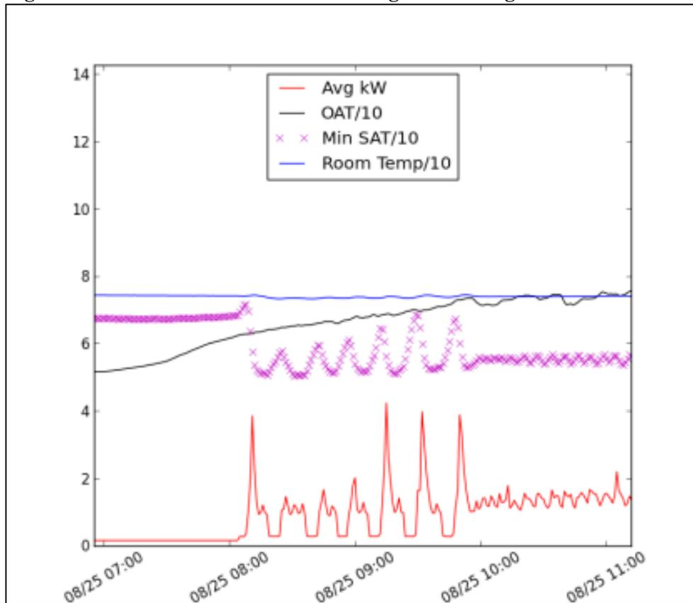
The argument for using the compressor during economizer cycles is rooted in the fan power laws. During the economizer interval, the airflow was low because the fan power was only about 120 W. At this low airflow, economizer operation is inherently limited. The RTU could have achieved more economizer-only cooling simply by increasing the airflow, but this would have increased the fan power significantly, probably to a level even higher than compressor energy.
