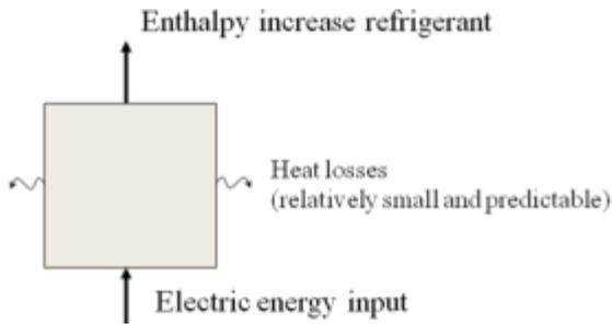
**Figure 22, The energy balance with consideration of heat losses over the compressor allows calculation of mass flow**
