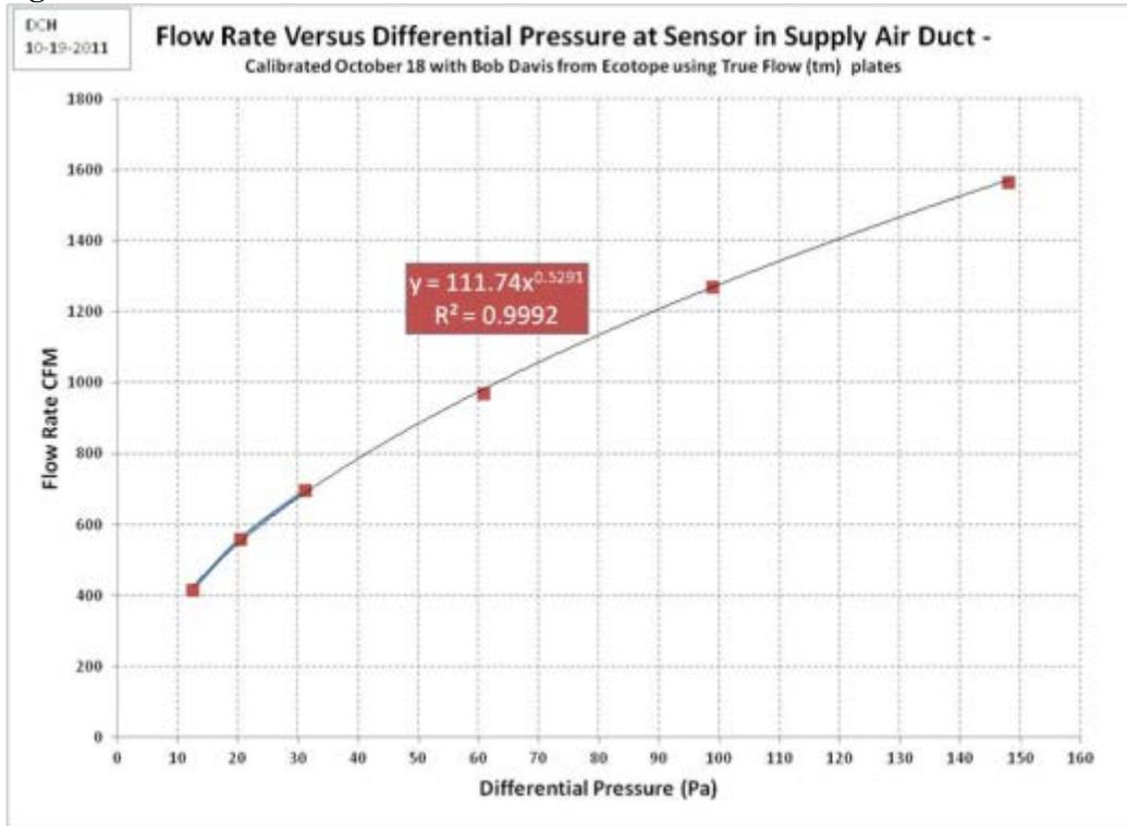
Figure 42. Calibration Curve for the Daikin Field Flow Measurement
