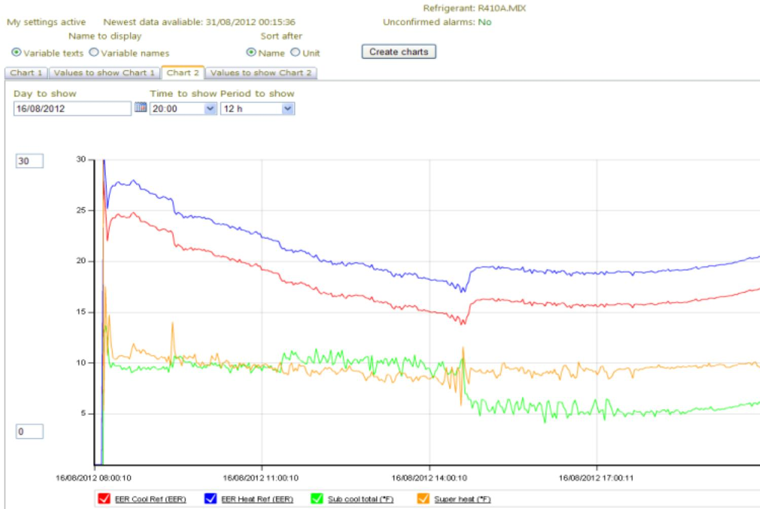
Figure 13, RTU2 superheat and sub cool (°F)
