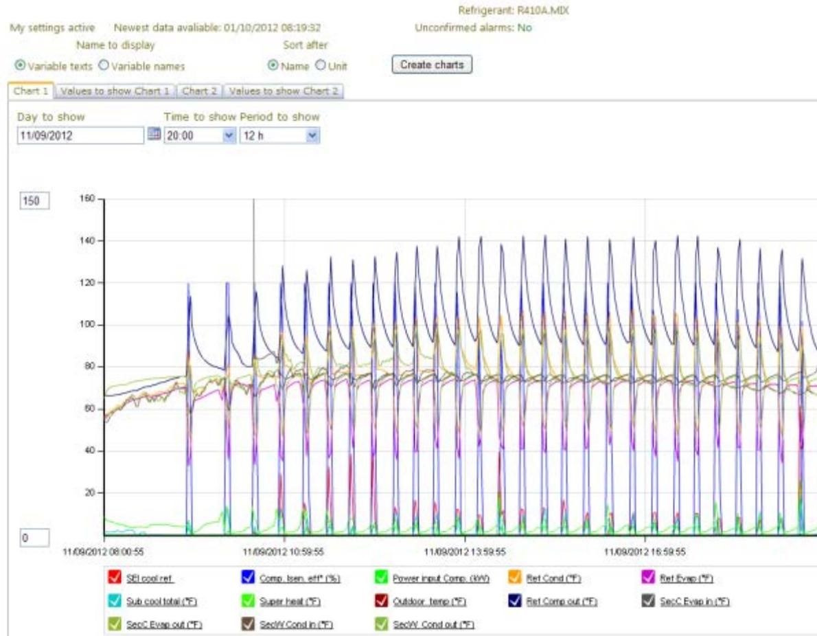
Figure 17, RTU3 on-off operation (°F)
