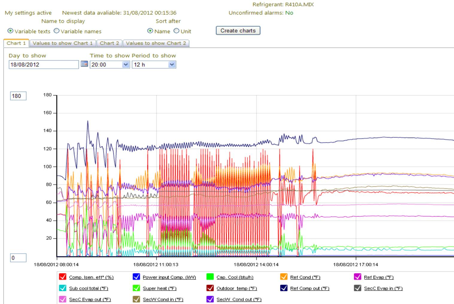
Figure 14, RTU2 excessive short cycling at low load and low ambient (control issue resolved)
