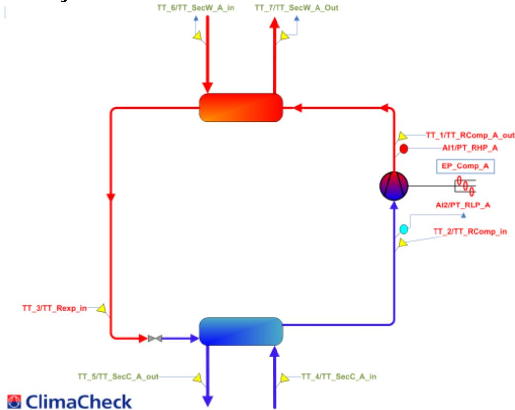
Figure 8, Standard sensor mounting
