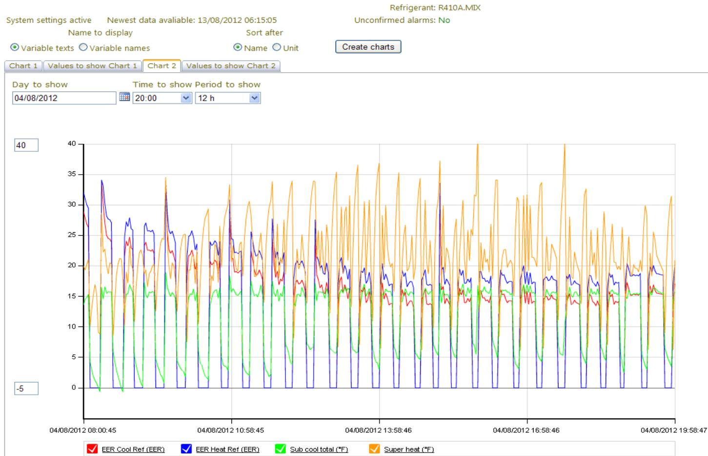
Figure 10, RTU1 Super heat and sub cool during On-Off operation (°F)
