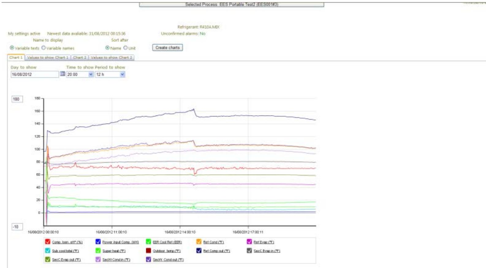
**Figure 12, RTU2 Control following change in ambient condition showing also change of condenser behaviour 14:40 (°F)**
