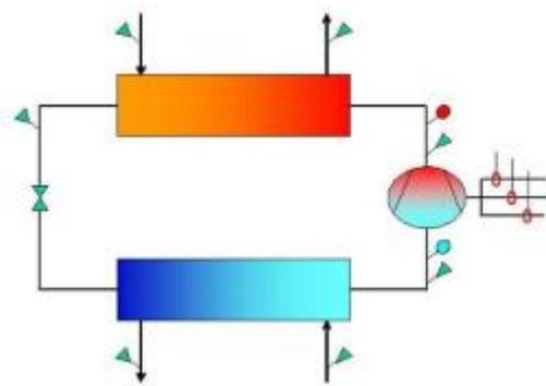
**Figure 21, Sensors required and their location to establish performance of a standard refrigeration system**
