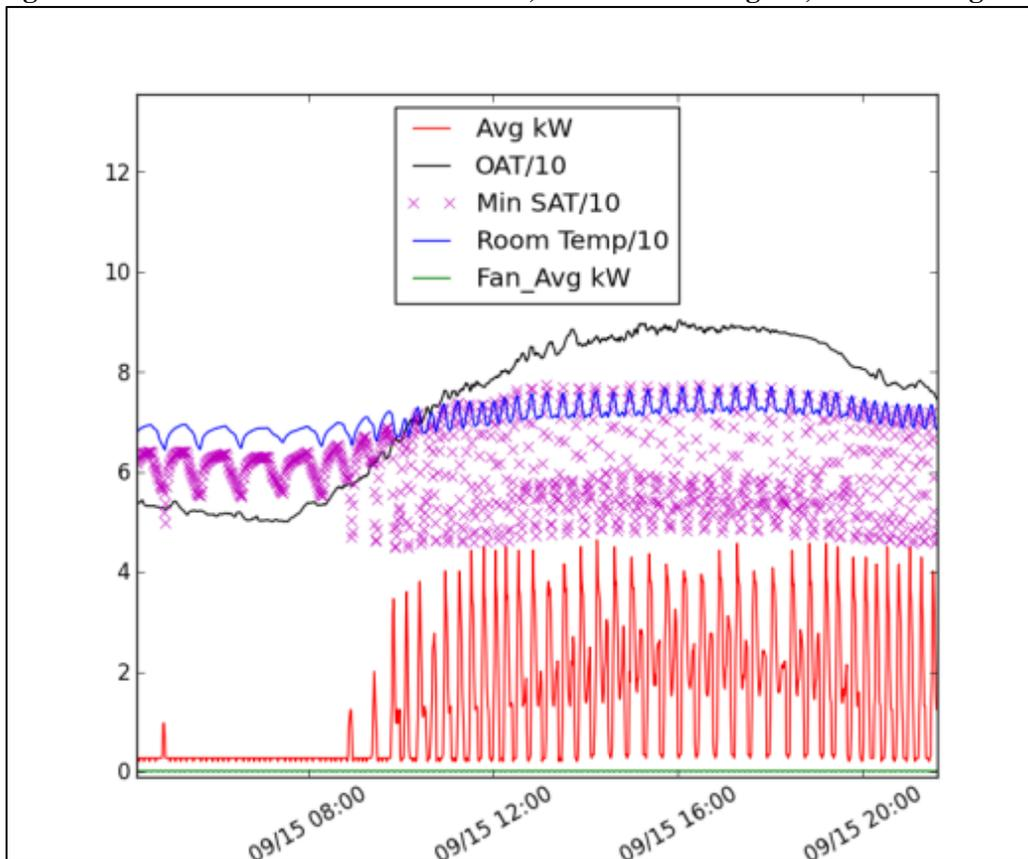
**Figure 31. Daikin One-Minute Time Series, ID-2 Control Regime, Field Testing**
