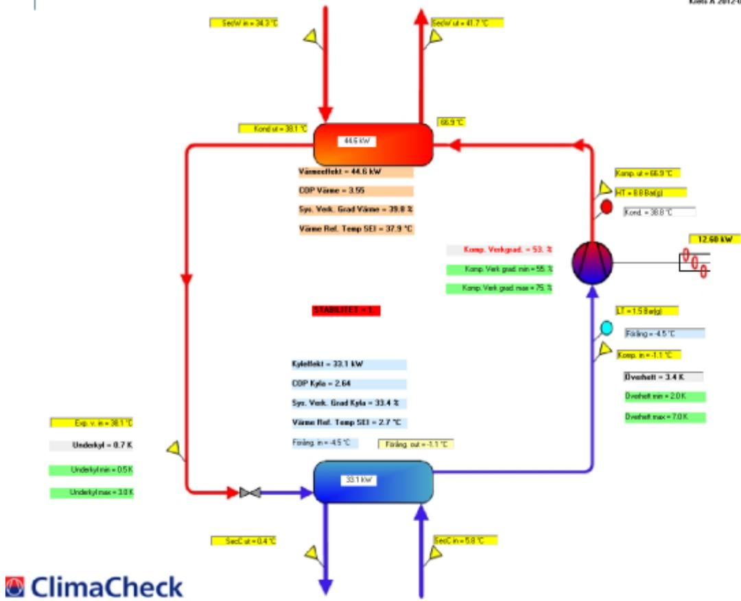
Figure 1, Flow chart of tested system
