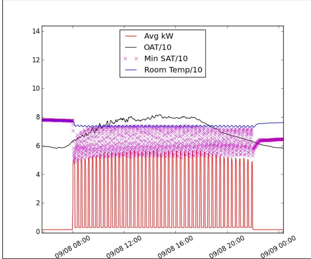
After a service call by Wytek personnel, researchers/Wytek personnel adjusted the economizer and fan controls. Figure 26 offers an example of the unit's operation during this A-3 regime. Inspection of the data shows that the economizer is now functioning, shown as a brief dip in power in the first cycle. The fan speed during ventilation is unchanged from A-2, with a minimum power of approximately 0.3 kW; however, the fan speed during compressor operation was reduced.
