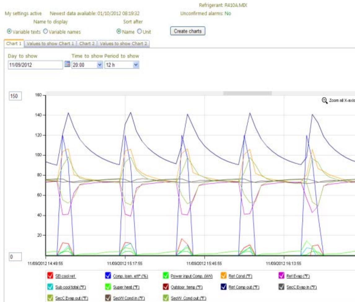
Figure 18, RTU3 sequence of short cycles (°F)
