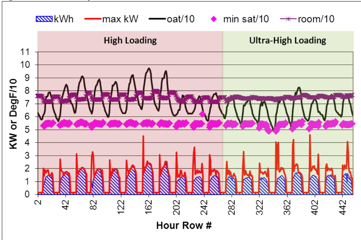
Figure 18 shows the one-minute time series for the Daikin unit. The modulation of the compressor is continuous throughout the cycle.
