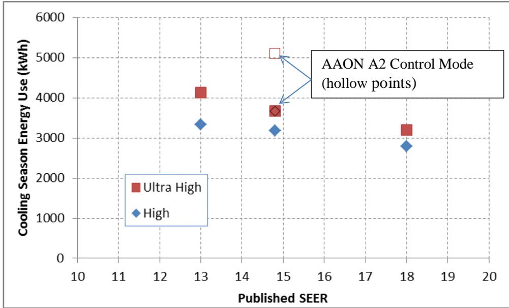
Figure 32 shows a comparison of the seven-day cooling season energy use projections for each unit versus the published SEER. Notably, increasing SEER and decreasing projected energy use appear to be correlated. However, when researchers made controls changes that resulted in very high compressor fan speeds (mode A2 shown by the hollow points), the correlation became much weaker.
