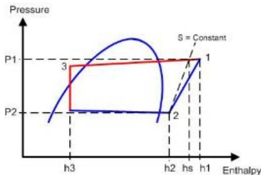
**Figure 23, Pressure – enthalpy graph of “standard” refrigeration process**
