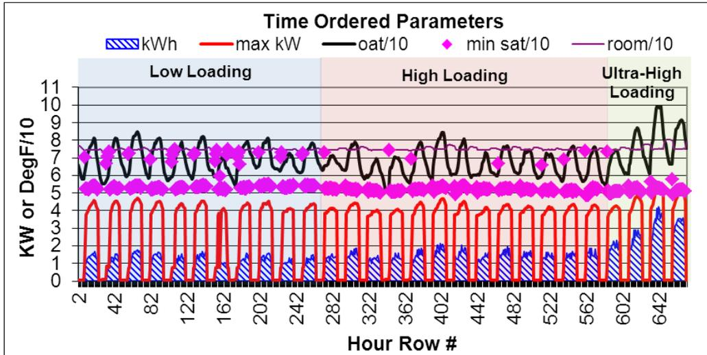
Notes: The air temperature points are divided by 10 so that the points fit on a single Y-axis. “OAT” represents outdoor air temperature; “min SAT” is the lowest supply air dry bulb temperature seen in the hour; and “room” is the test space dry-bulb air temperature.
