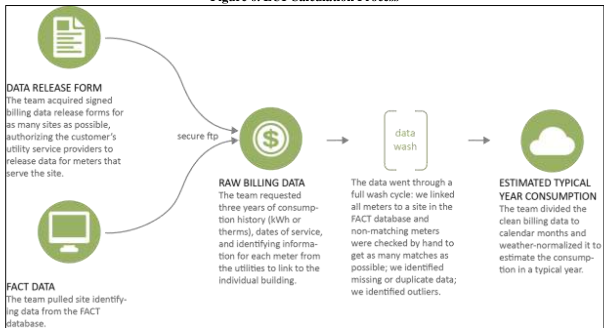
Figure 6. EUI Calculation Process
