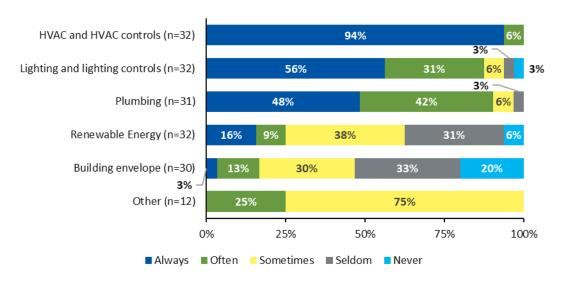
Figure 4. Frequency of Commissioning by Equipment/System Type During New Building Commissioning
