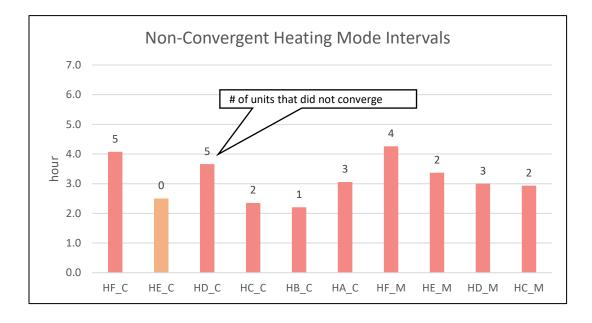
• As the building load increases, the main contributor to the non-convergence transitions from irregular ON/OFF cycling to a combination of irregular ON/OFF cycling & defrost operation to defrost operation. This pattern occurs in both sets of test intervals (marine and continental).
