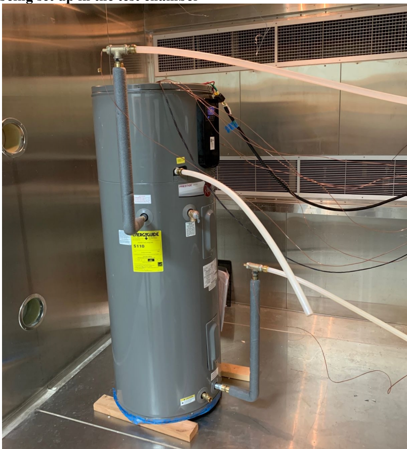
Figure 2. Generation 5 Premium (Gen5p) 50-gallon HPWH being set up in the test chamber
