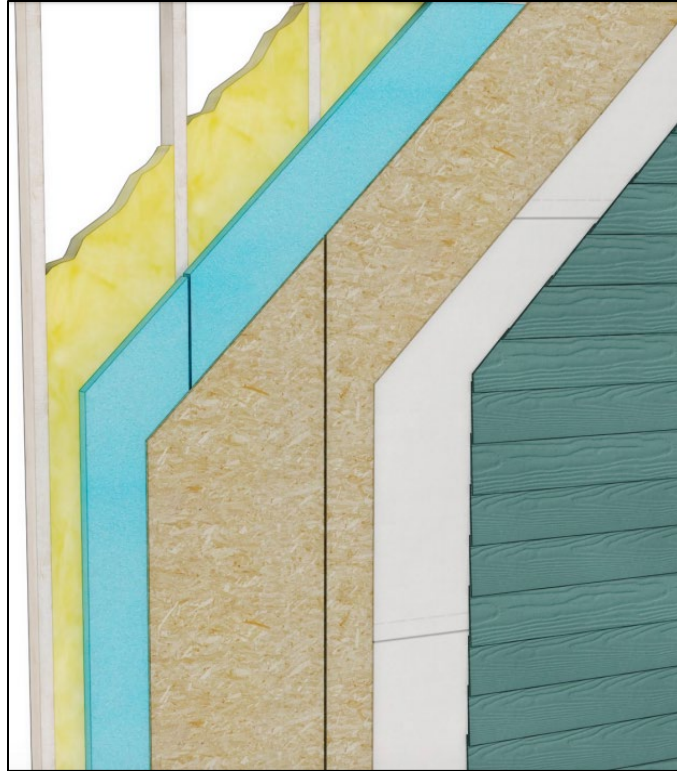
Figure 8. Exterior View of Staggered Layers to Minimize Seam Alignment. Courtesy of Home Innovation Research Labs (Gunderson & Kochkin, 2018)
