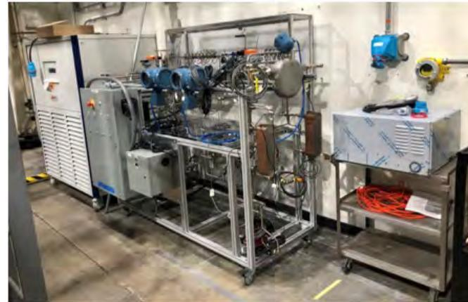
Liquid-to-refrigerant heat exchanger test facility
