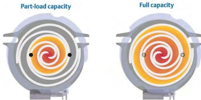
Improved from 2-stage compressor using mechanical capacity modulation
