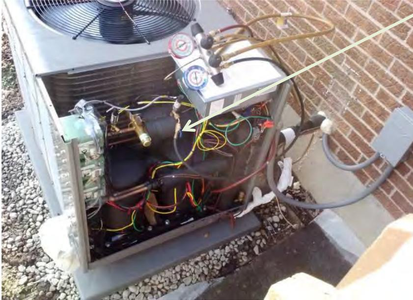
Field testing in OH-outdoor unit, at a residential home having a design cooling load of 3-ton (10.6 kW)
