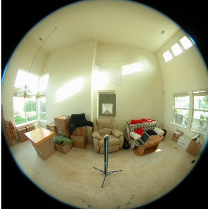
Figure 8 – Fisheye photo of test space. The windows at left face west, those at right face east. Note the ALDI mounted on a tripod 3' in front of the lens.
