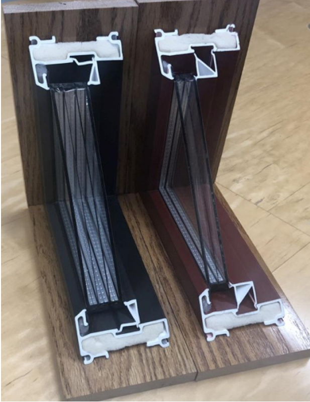
Figure A5-6 Photos of two window corner samples showing a quad unit (l) and a triple unit (r); the quad unit utilizes a 1 ¼" wide IGU and can be optimized to achieve ~R15 COG ( Courtesy Alpen)
