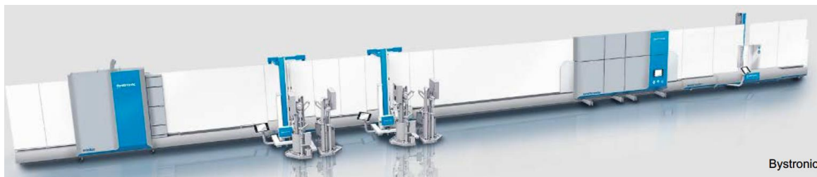
Figure A3-5 : Example of Automated IGU Assembly Line ( source: Bystronic)
