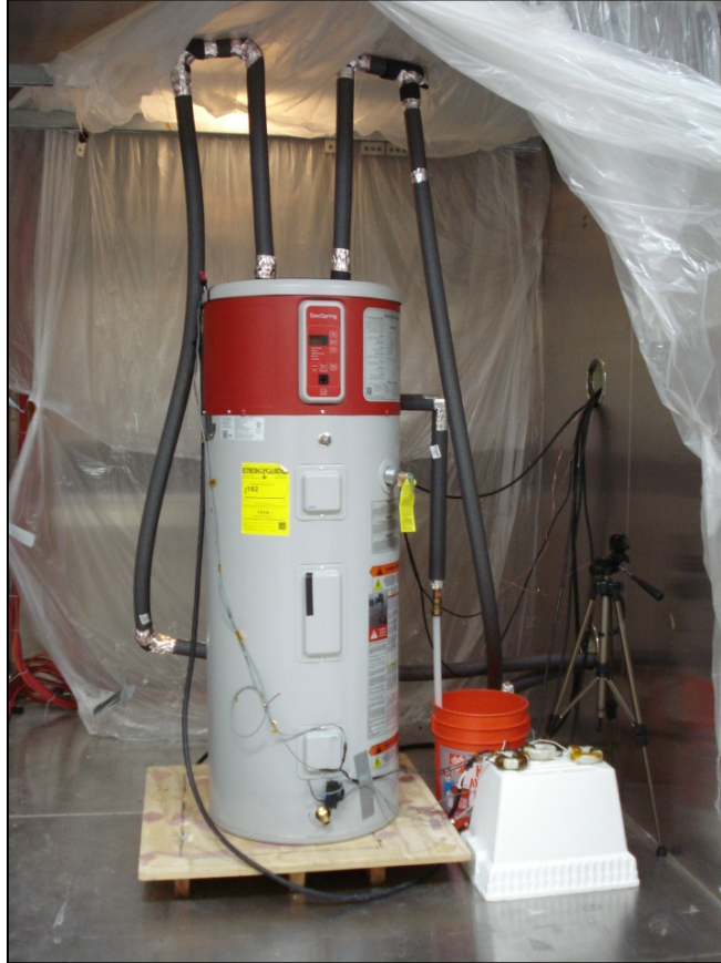
Figure 1. HPWH Test Unit Installed Inside Thermal Chamber
