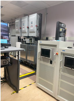
PSU PEG Invert Testing Bays (L) Grid & Load Simulators (R)
