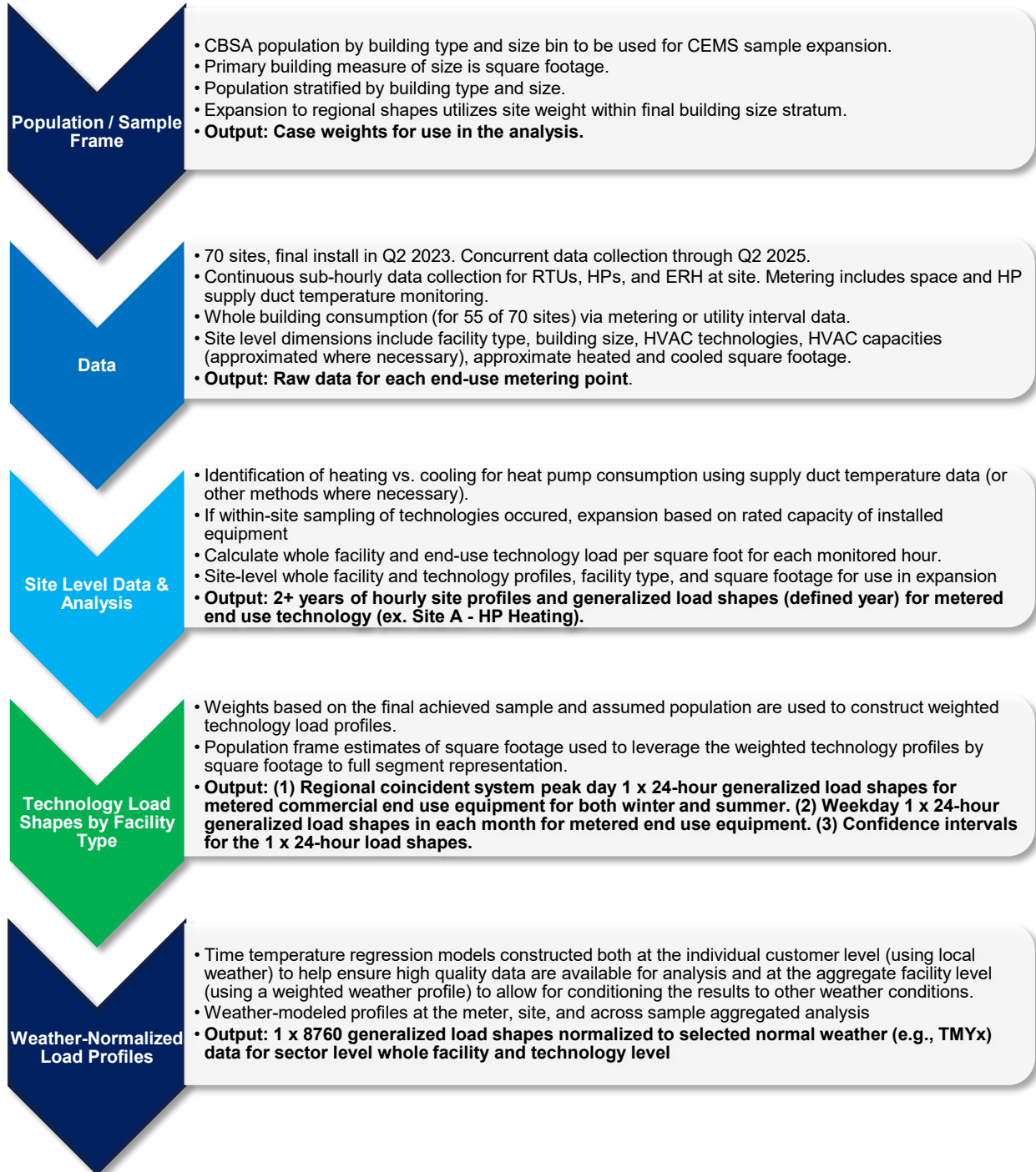
Figure 2-1. Overview of analysis approach
