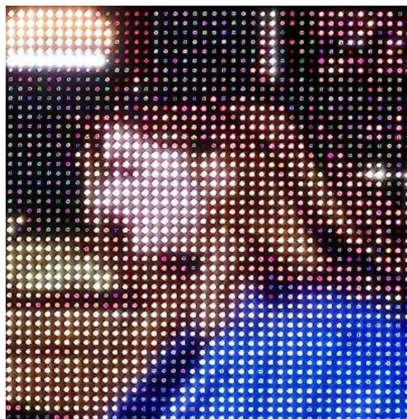
Figure 84: DVLED displays control light emission at a sub-pixel level
