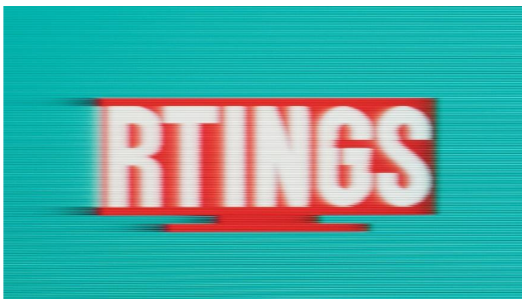
Figure 64: The dark trails that the moving logo leaves behind are an example of ghosting from RTINGS
