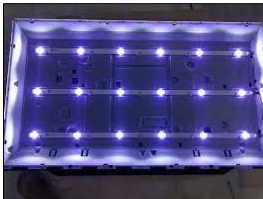
Figure 1: A 3x6 LED direct-lit backlight array
