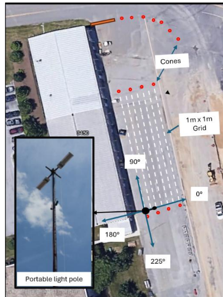
Figure 1. Plan-view definition of pole placement and sensor orientation relative to the fixed experimental grid.
