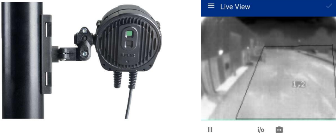
Figure 21. TrafiOne 195 sensor (left) and example software-defined thermal detection zone (right).
